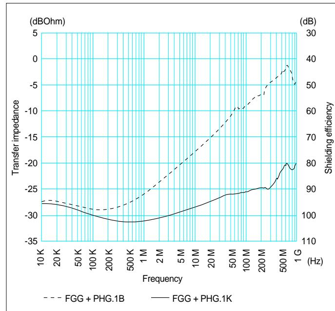
The performance of S and B series connectors is comparable to the results of measurements carried out on a pair of FGG + PHG.1B connectors.
