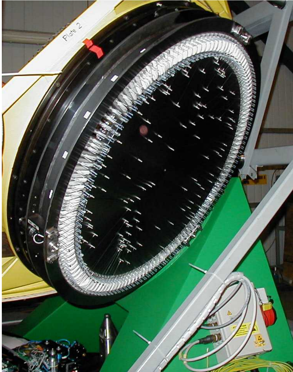
Figure 3.2: One of the two plates of the fibre positioner OzPoz. The fibres are attached to the plate using magnetic buttons.
