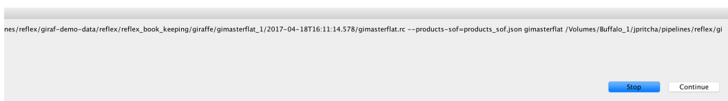
Figure 8.2: If the MasterFlat recipe fails, a ridiculously wide error message window like the one above will popup, once mouse-click-dragged to the left you will discover the Stop and Continue buttons. Click the Continue button and the Interactive MasterFlat GUI window will open, see figure 8.3.
