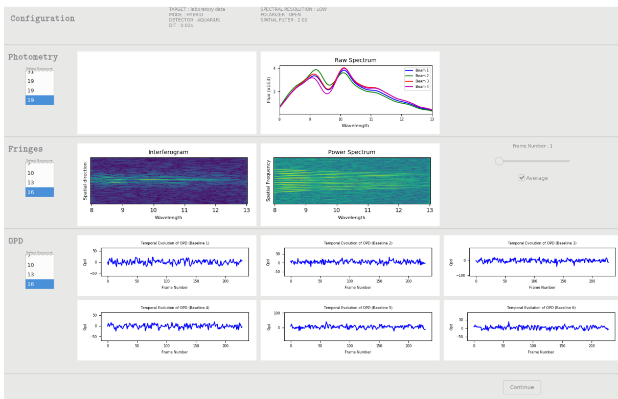
Figure 9.3: The MATISSE interactive plot window for reduced N-band data. Note that here, in low spectral resolution, the entire N-band wavelength range is displayed. The photometry plot is empty as no simultaneous photometry is recorded during fringe tracking in the N band.
