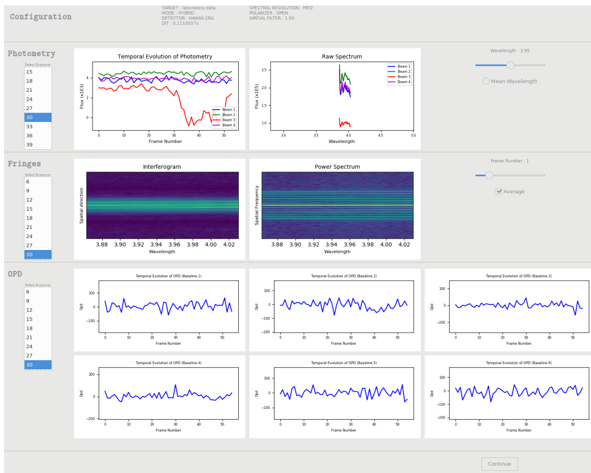
Figure 9.2: The MATISSE interactive plot window for reduced LM-data. Click in the boxes on the left side to select specific exposures (TPL.EXPNO) Note that here the medium spectral resolution was specified in the OB, so only a rather small wavelength range is displayed around the specified central wavelength. Despite a brief drop-out in flux for beam three in the displayed exposure, not effect can be seen in the fringe and OPD panels. The OPD traces appear flat because fringe tracking was performed in the L-band.
