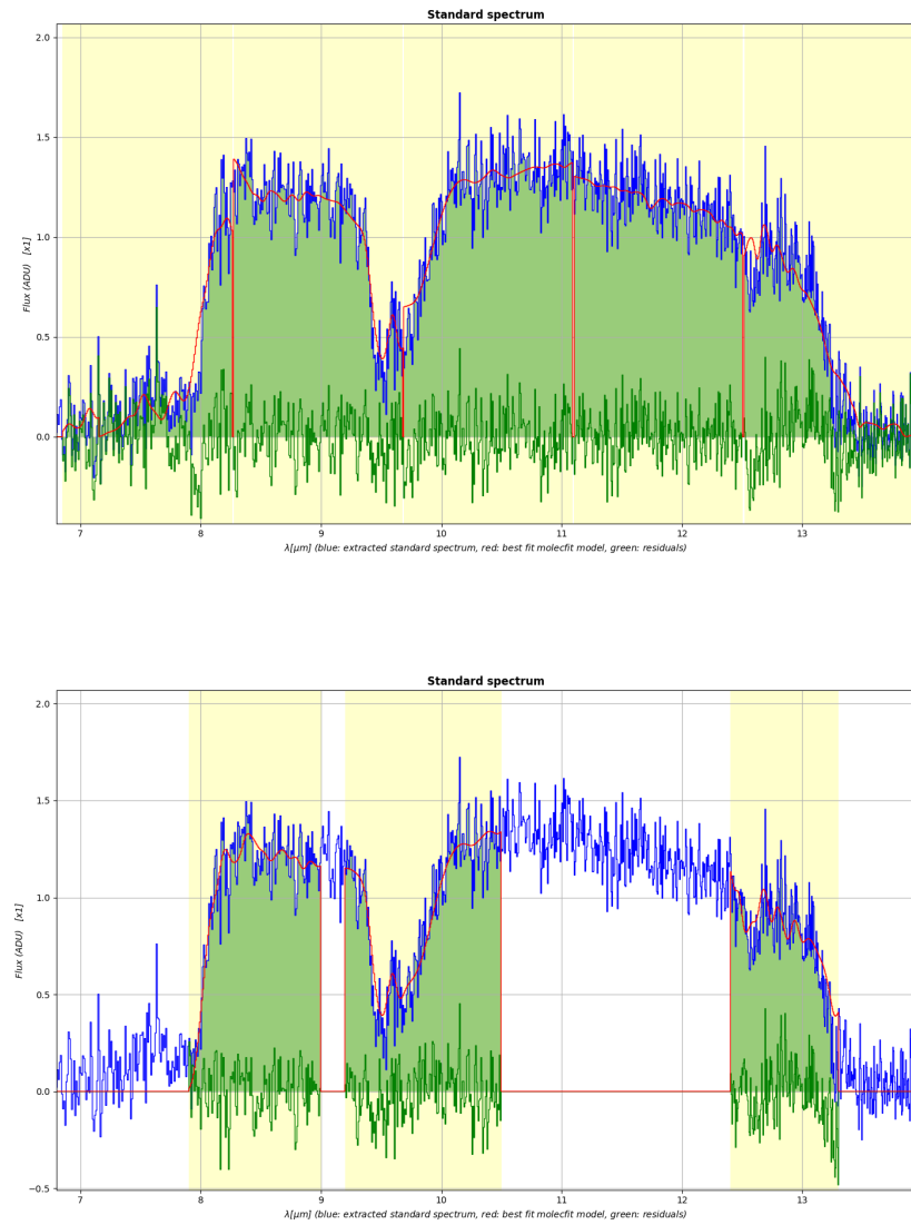
Figure 8.8: Upper panel: the result of the modeling step on the demo dataset SCI_SPC_Mrk926_SPC_OBS_LMR_TAB with default automatic parameters setup. Lower panel, as upper panel, but with the modified inclusion regions and molecules (see text for details).
