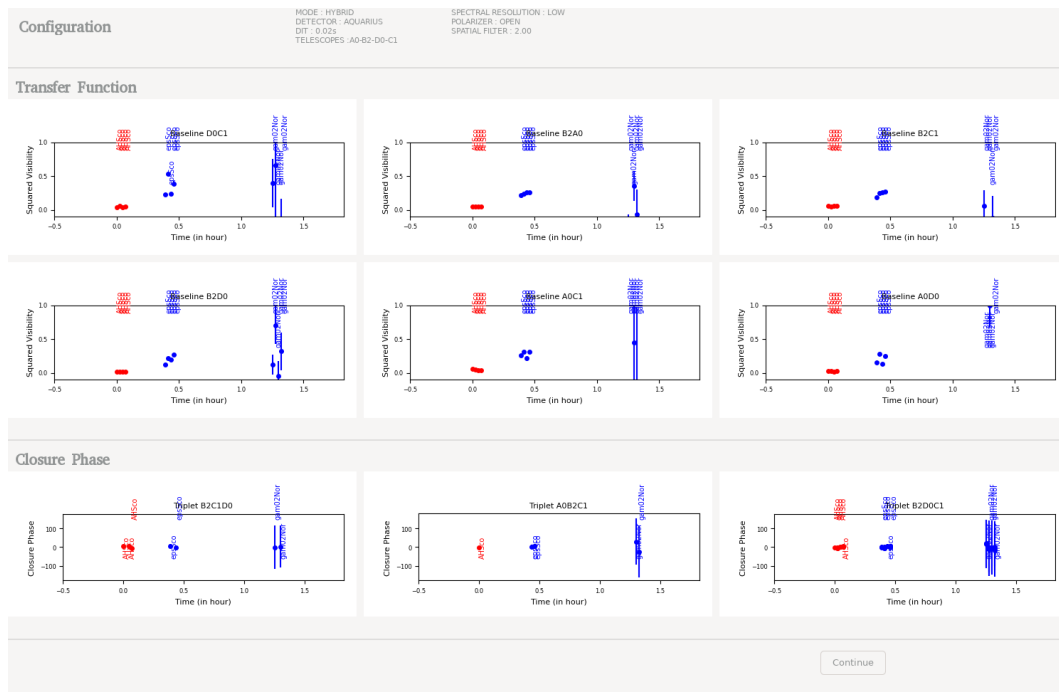
Figure 9.7: Transfer function (visibilities and phases uncorrected for the object structure/diameter) in the N band (first exposure). Note that the calibrator phases are near zero, but the amplitudes of both CAL and SCI are low due to instrmental loss of coherence. Here, the calibrator has a flux of 50 Jy in the N band, and was intended to calibrate the N band data only.
