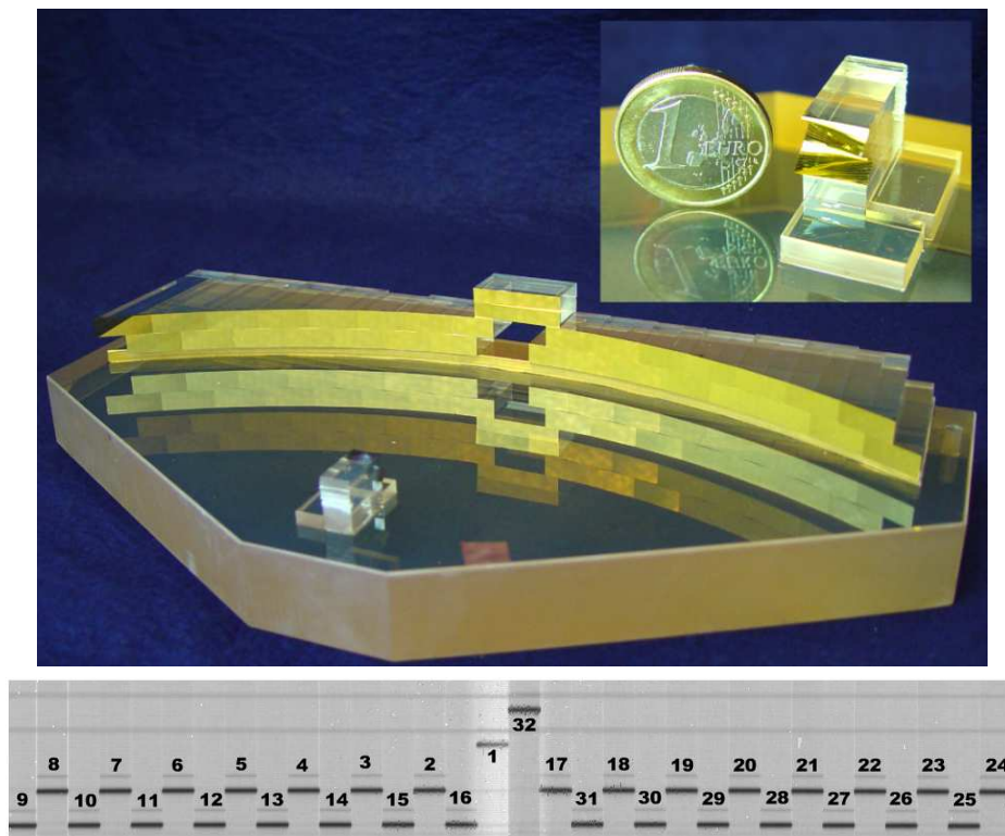
Figure 4.1.2: SPIFFI image slicer (top): The light enters through the hole in the big slicer. A stack of 32 small mirrors, the small slicer (also shown in the sub-panel), slices the image and redirects the light towards the 32 mirrors of the big slicer, which re-arranges the slitlets into a 31 cm long pseudo-slit. (bottom). The layout of the slitlets on a raw SPIFFI frame.
