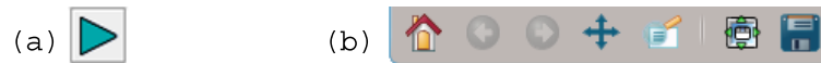
Figure 2: (a) ‘Run’ button to start the Reflex workflow; (b) zoom toolbar provided by the Python library matplotlib . With the leftmost symbol, the user always comes back to the overview; the second and the third symbol enables the user to go ‘Back’ and ‘Forward’ in the zooming history; the 4 th button shifts the plot via the mouse; the 5 th button is the actual zooming button, which can be used via the mouse; the 6 th button opens a window to configure the subplots; the 7 th button saves the plot to a file.
