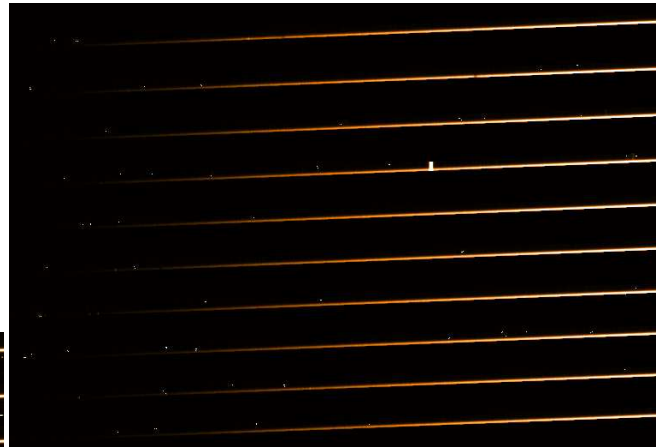
Figure 11.1.6: Science image reconstructed from the extracted spectra and cosmic ray map. For illustration purposes only the spectrum was extracted using a short slit (1/4 of full slit) with a small positive offset (+1/8 of full slit). This reconstructed image shows the locations of the detected cosmic rays, the sky emission line, and that the overall spectrum shape is very similar to the input spectrum. Of course, regions outside the specified extraction slit are not “seen” by the extraction algorithm and are therefore black.
