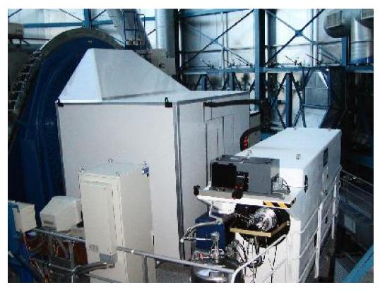
Figure 4.0.1: A photo of FLAMES mounted at the Nasmyth A focus of Kuyen (VLT-UT2).
