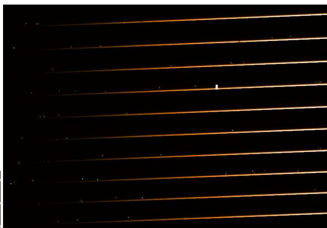
Figure 11.1.6: Science image reconstructed from the extracted spectra and cosmic ray map. For illustration purposes only the spectrum was extracted using a short slit (1/4 of full slit) with a small positive offset (+1/8 of full slit). This reconstructed image shows the locations of the detected cosmic rays, the sky emission line, and that the overall spectrum shape is very similar to the input spectrum. Of course, regions outside the specified extraction slit are not “seen” by the extraction algorithm and are therefore black.
