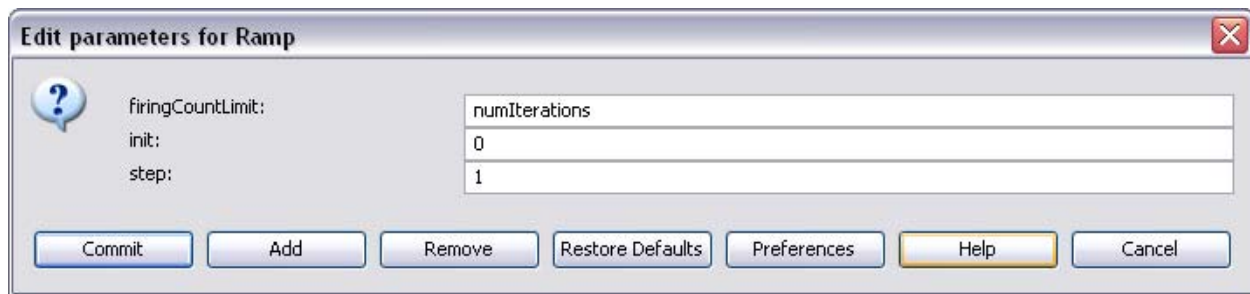
Figure 38: The Ramp actor parameters from the prototype ENM Calculate Omission/Commission sub-workflow. The firingCountLimit is set to the value "numIterations", which is defined as 10 by a workflow parameter.
