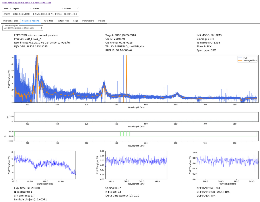
Figure 20: The quality plot (graphic report) associated to the tasks object and rv_stars , showing the extracted spectrum (S1D_FINAL_A) and zooms on selected regions. A smoothed version of the spectrum is also shown.
