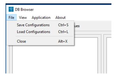
Saving and loading configurations is a very simple process that requires the user to specify the JSON file where the configurations are going to be saved or loaded from. During this process a typical window, as depicted below, will appear when selecting any of the configuration options.
