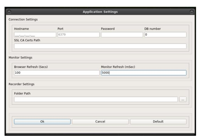
In the **Connection Settings** section, all of the configuration parameters required to establish a REDIS connection can be found.
