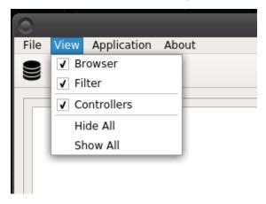
A "Hide All" option is also present, which can be very useful, in those cases where a stripped down version of the application is required, either because the list of monitored elements is static, i.e. the list don't change over time, or when running multiple applications simultaneously and side-by-side is required. Below it is possible to see the stripped down version of the application layout. To quickly return to the default view, a "Show All" option is present as well.
