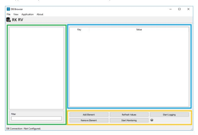
The Browser component, located on the left side of the application, is composed by two functional elements: a list widget and a filter field. The list widget provides the necessary support for displaying the existing keys for a given database.
