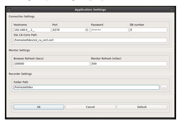
At the **Monitor Settings** section, the user can specify following parameters:
