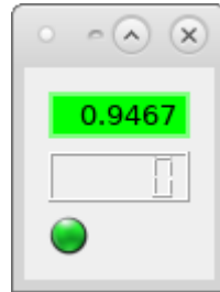
Fig. 33: Display widgets, from top to bottom TaurusLabel, TaurusLCD and TaurusLed
