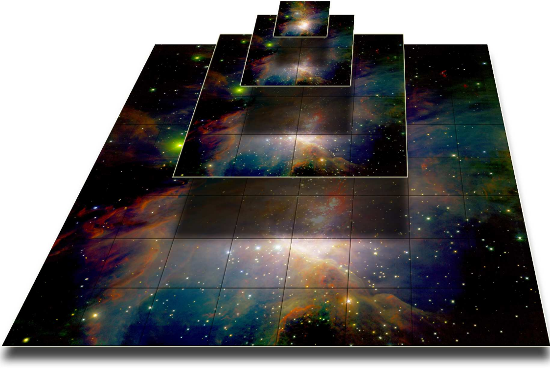
Figure 7: Depiction of a tiled, four-level image pyramid (Orion nebula observed with the WIRCAM instrument, picture credits CFHT/C.Marmo/Terapix).
